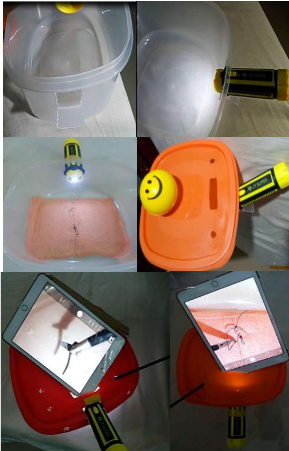
Figure 3. Making of Flap for LED torch and placement of stress ball,I pad and instrument
